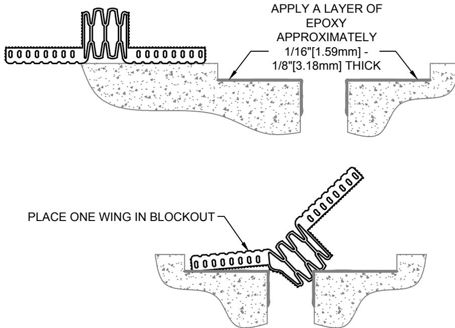
**\*IMPORTANT NOTE:** Do not use Epoxy or install this seal if either the substrate temperature or air temperature will drop below 40°F [5°C] during the installation or cure time of 8 hours.
